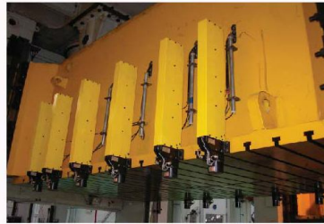
Auto-Travelling Hydraulic Clamp 自走式油壓夾貝
